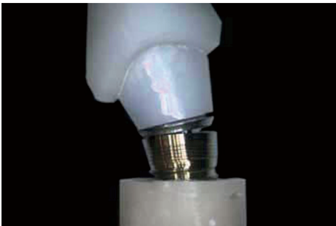
12 Representative specimen displaying severe distortion of test implant of Lava abutment.
