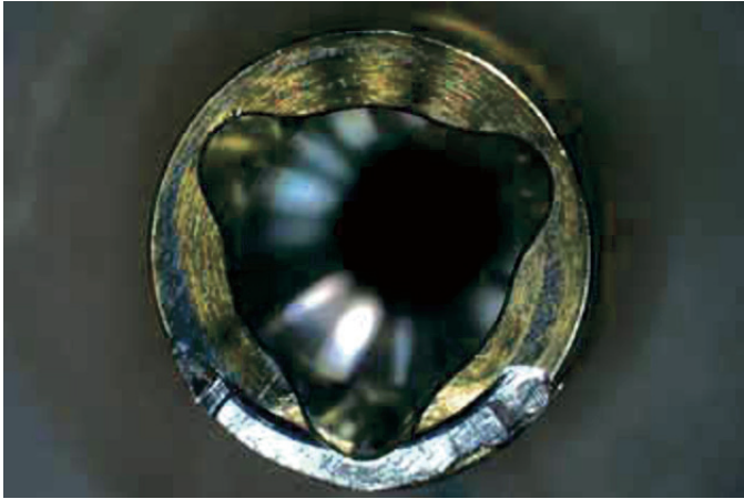
10 Representative specimen displaying damage to implant platform of Procera abutment.
