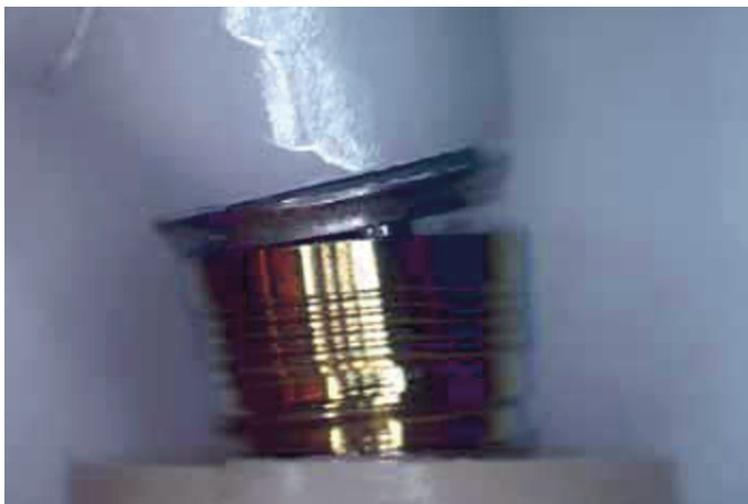
8 Lava abutment displaying separation between zirconia and titanium insert.
