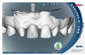
Figure 2a. Facial view of a scanned definitive cast with a designed CAD/CAM abutment for a cement retained implant-supported crown. The design is based on the contours of the superimposed model of the provisional restoration, ensuring adequate support of the soft tissue and space for the prospective restorative materials.
