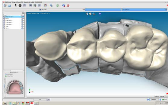
Figures 1a and 1b. Occlusal view of a scanned definitive cast prepared for a bilayered zirconia-based crown on the canine, a fixed dental prosthesis with a monolithic zirconia design on the molar retainer, and a hybrid design on the pontic and premolar retainer.
